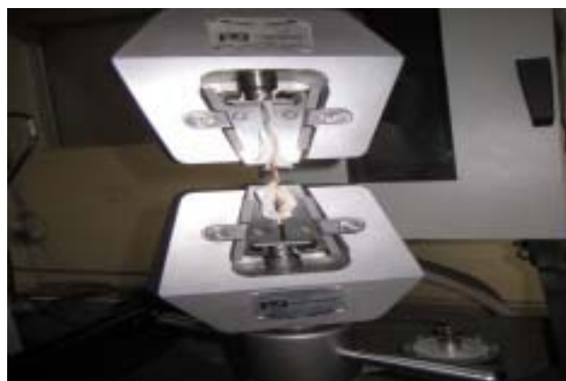
Fig.10. Tensile strength measurement by universal testing machine (Instron-3382).
